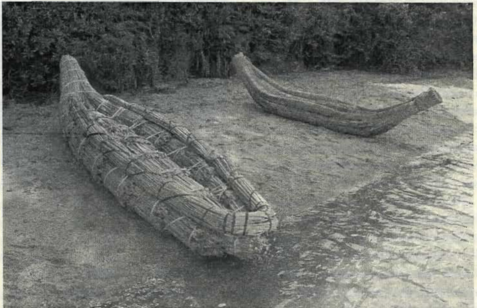
A Pomo-style tule boat bound with split maple shoots and bark (left) and a Bolivian-style tule boat, constructed by MAPOM's Charles Kennard, rest on the shore of Tomales Bay. photograph courtesy of Charles Kennard
